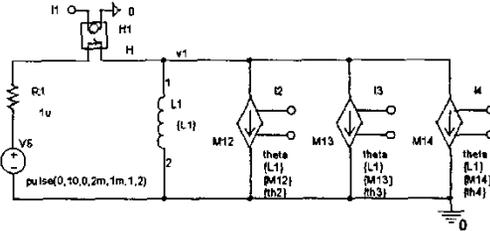
Figure 3. PSPICE equivalent circuit for rotor winding coupled to three-phase armature winding.
