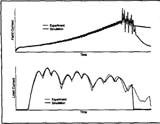
Figure 2. Results from the simulation comparing the field current (top) and the load current (bottom) for shot SC398 on the SSFTP system. Note that the time scales on the two plots are different.
