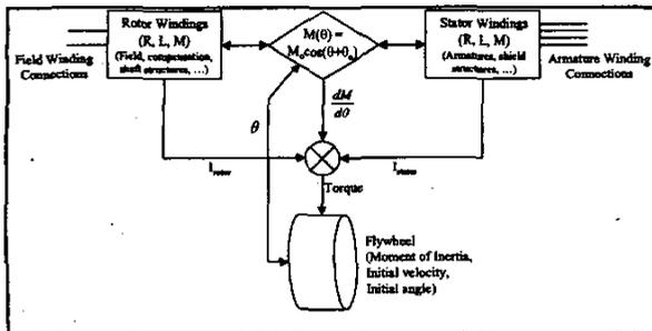
Figure 1. Block diagram layout of pulsed alternator model.
