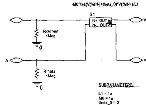
Figure 4. PSPICE sub-circuit for the dual input current source representing angular-dependent mutual coupling.
