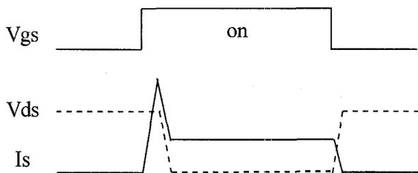
Fig. 2 Power Switch Switching waveforms
