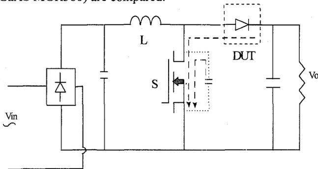
Fig. 1 Hard -Switching PFC boost converter
