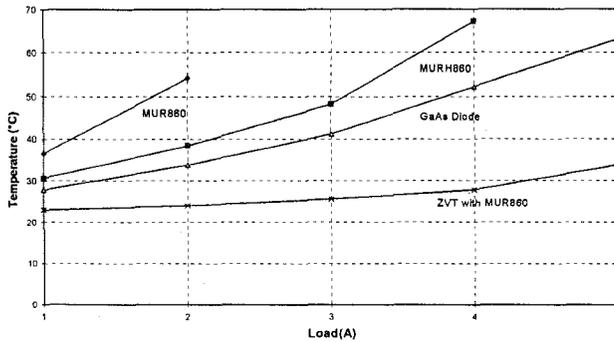
Fig. 7 Temperature of the Power Switch ( $V_o=400 V$ )
