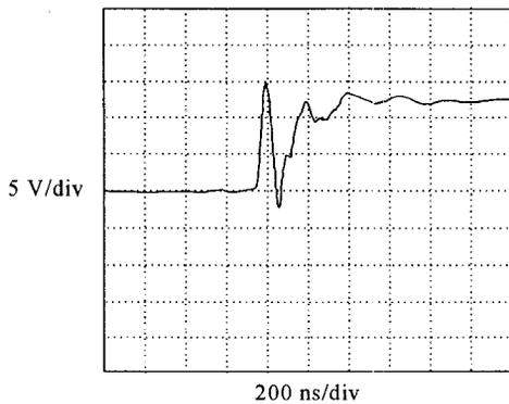
Fig. 16 Turn-On Gate Signal Waveform
