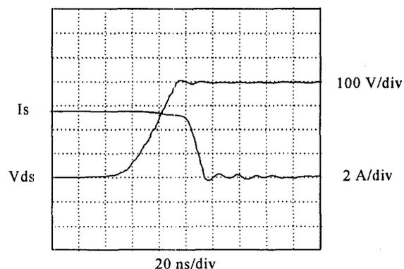
Fig. 12 Hard-switching with the MGR560 Power Switch Turn-off ( $V_o=400$  V,  $I_o=5$  A)
