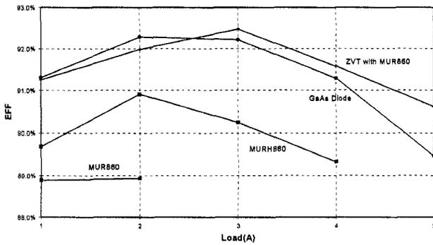
Fig. 6. Efficiency Comparison ( $V_o=400V$ )
