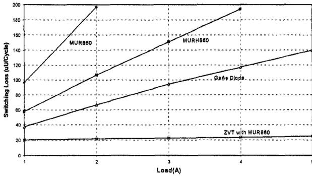
Fig. 5 Switching Loss of the Power switch ( $V_o=400V$ )
