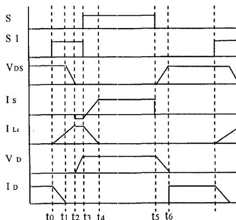
Fig. 4 Key waveforms in the ZVT Circuit
