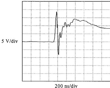
Fig. 17 Turn-On Gate Signal Waveform
