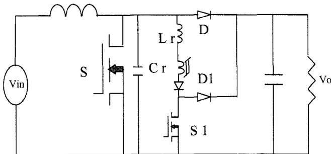
Fig. 13 The ZVT Circuit Used in Test
