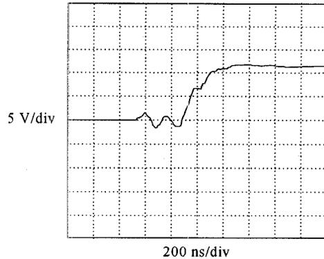
Fig. 19 Turn-On Gate Signal Waveform
