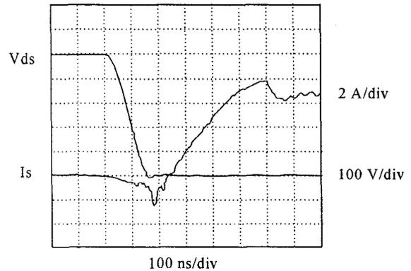
Fig. 14 ZVT with the MUR860 Power Switch Turn-On ( $V_o=400$  V,  $I_o=5$  A)
