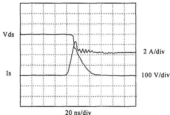
Fig.10 Hard-Switching with the MURH860 Power Switch Turn-On ( $V_o=400$  V,  $I_o=4$  A)
