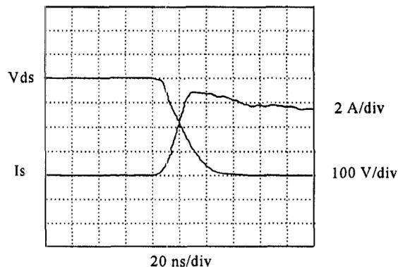
Fig. 11 Hard-switching with the MGR560 Power Switch Turn-On ( $V_o=400$  V,  $I_o=5$  A)
