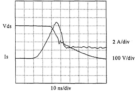
Fig. 9 Hard-switching with the MUR860 Power Switch Turn-On ( $V_o=400V$ ,  $I_o=2 A$ )
