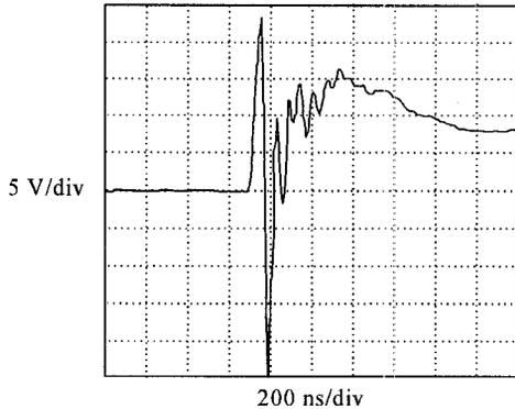
Fig. 16 Turn-On Gate Signal Waveform
