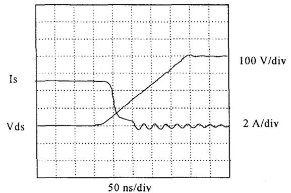
Fig. 15 ZVT with the MUR860 Power Switch Turn-Off ( $V_o=400$  V,  $I_o=5$  A)
